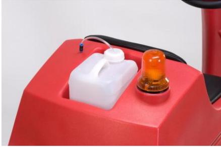
*Chemical canister integrated in the machine*
